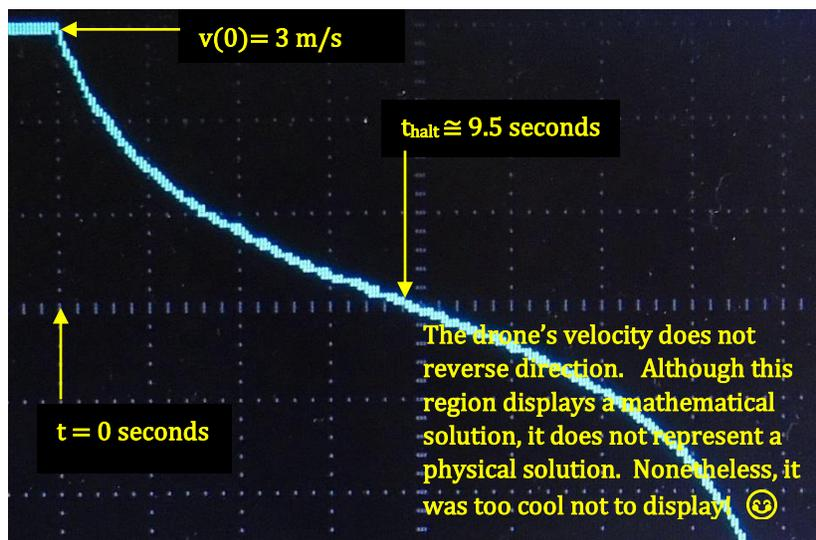
Figure 3: Drone speed as a function of time\*
