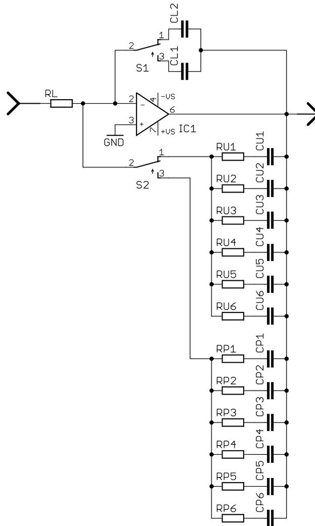
Figure 1: Basic circuit for the simulation of neutron kinetics with six groups of delayed neutrons
