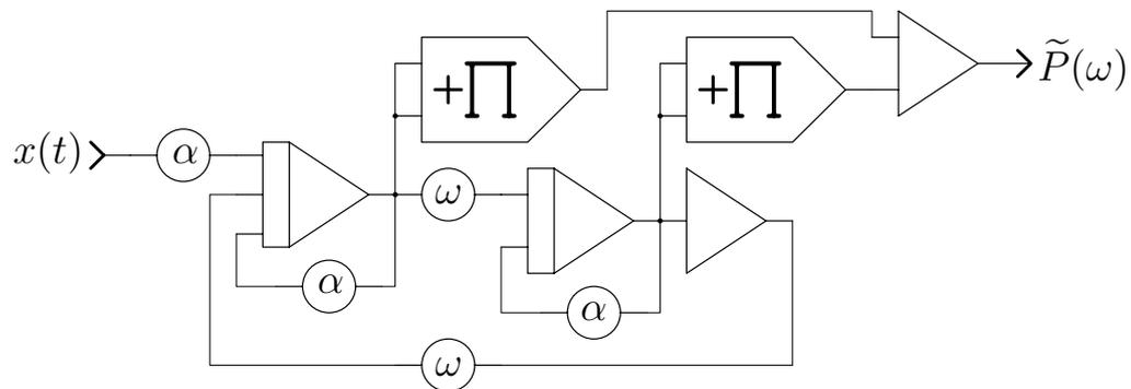
Figure 4: EMP FOURIER circuit
