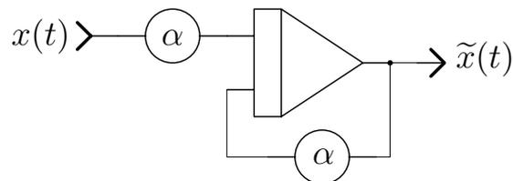
Figure 1: EMP mean circuit – the parameter  $\alpha$  determines how quickly the weighing function “forgets” past input values
