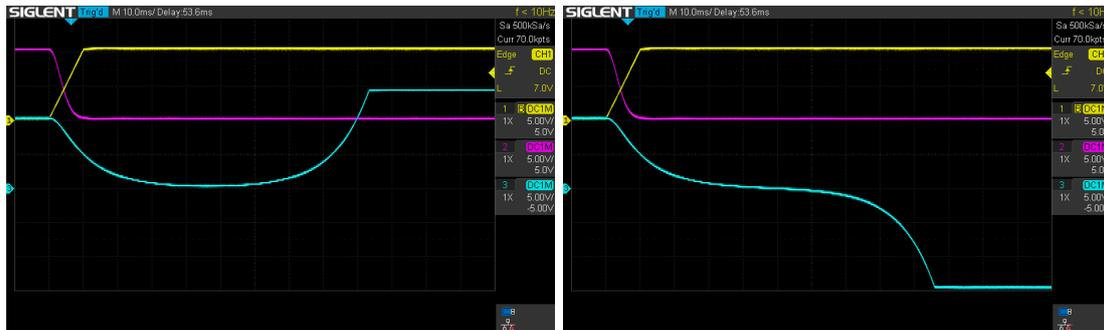
Figure 3: Two runs of the analog program for  $E = -0.1$  and  $\alpha = 0.1$  with  $\alpha t$  in yellow,  $f(t := \sqrt{\frac{2}{\alpha}}\xi)$  in red and  $\psi(t := \sqrt{\frac{2}{\alpha}}\xi)$  in blue. The potential depth is  $v_0 \approx 0.342$  for the left run and  $v_0 \approx 0.343$  for the right run.
