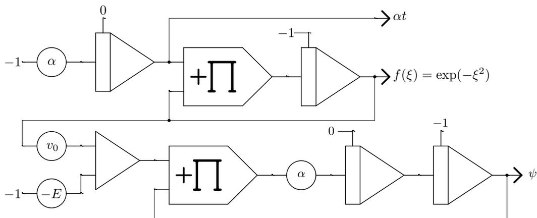
Figure 2: Analog computer program solving the SCHRÖDINGER equation with GAUSSIAN potential.
